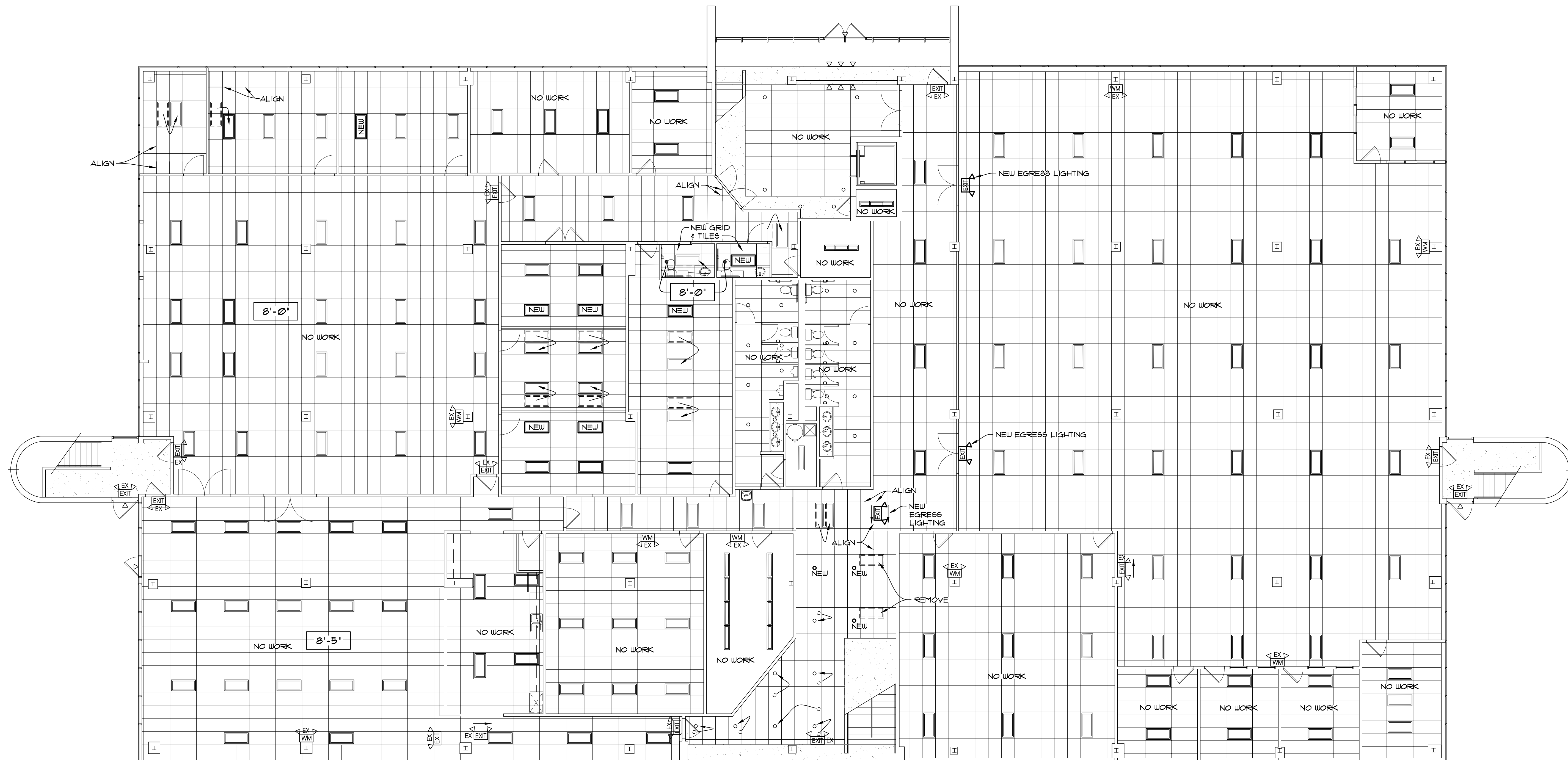
1 FIRST FLOOR REFLECTED CEILING PLAN A4 1/8" = 1'-0"
